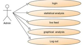
Fig.2 Interaction between Admin and Analytical Server (Use Case ID 1)
