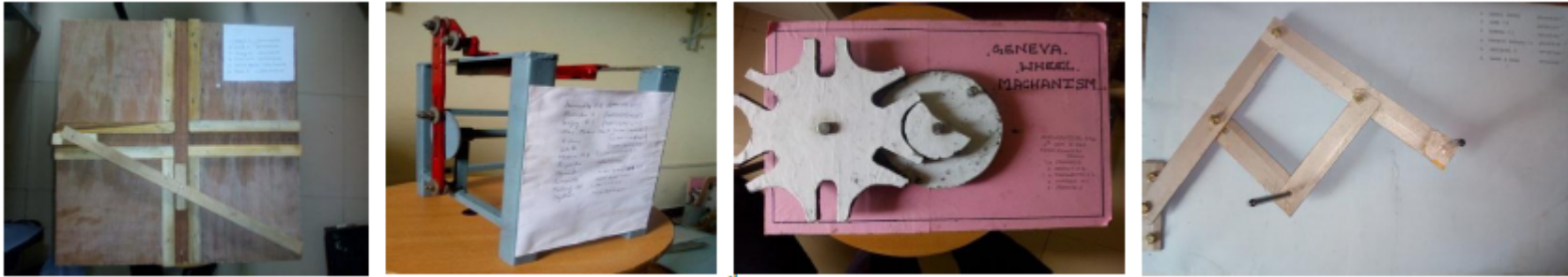
Figure 5.4: Working Models of Elliptical Trammel, Quick Return motion mechanism, Geneva Wheel Mechanism, Rat chat and Pawl Mechanism, Crank-crank mechanism
